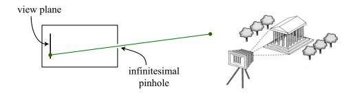
Light from a point travels along a single straight path through a pinhole onto the view plane. The object is imaged upside-down on the image plane.
